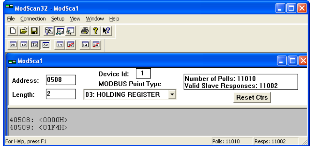
Figure 3-10: Modbus - configuration example 4 - active power
