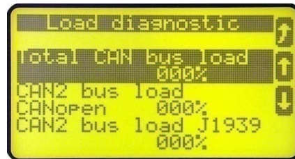
Figure 2-1: CAN bus load diagnostic screen
